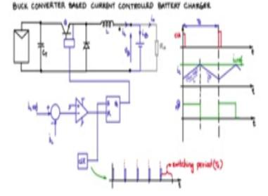
The inductor current here what we have drawn during 1-DTS period during the time and the switches of the slope of the inductor current is - V0 /L on -VB/L on the magnitude of that slope is VB/ L so this inductor we by the faraday equation the VL voltage cross the inductor is given by L DIL / DT.
