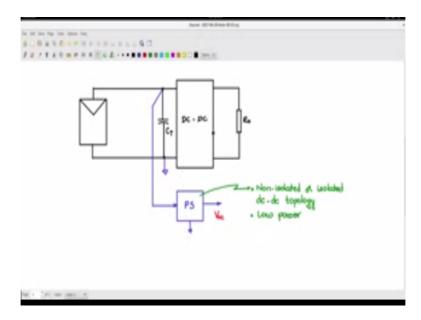
Consider this PV source and the DC-DC power supply which is acting as a interface between  $R_0$  and the PV source. You have above the capacitor CT and across the buffer capacitor CT let us tap of a line, and let us draw the input for the power supply from here. So this will act as the input to the power supply circuit, so PS is the power supply circuit which will deliver some output.
