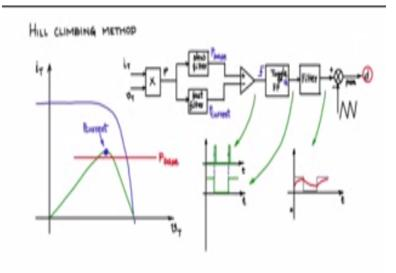
We shall now discuss the hill climbing method for maximum power point tracking. It is a very robust and popular method, it does not use the reference cell, it does not use sampling, it does not use any resistive switches there is no d/dt, no derivative terms only I and V terminal current and terminal voltage are measured, and based on the calculation of the power the hill climbing algorithm is used for tracking the maximum power point.
