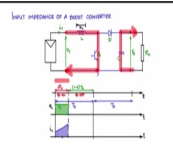
Let us see how we can use the boost converter as a power interface for MPPT consider this photovoltaic like module and this photovoltaic module is now interfaced to the load or not by a boost converter boost converter is having an inductance that is input I switch a power semiconductor switch like this now this could be a BJT as shown here or it could be an IGBT or it could be a MOSFET any of the switches any of the power semiconductor switches can be used herein switched mode on/off mode.
