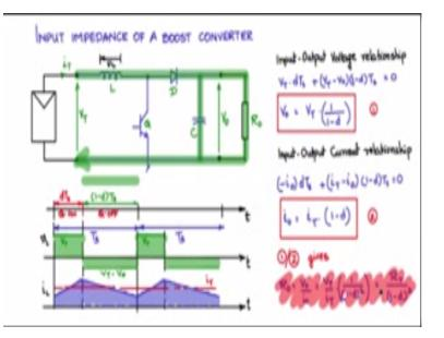
During the time when Q is off Q is off but the inductor current has to continue to flow so it will change polarity here and it will drive this diode on and charge up the capacitance and also the current will flow through the load and supply the load. So you will see that the inductor the stored magnetic charge in the inductor will discharge both through the capacitor and the load.
