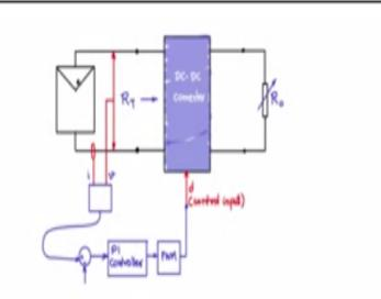
Let us see how we give this control input to the DC-DC converter in a generic way in such a way that  $R_T$  is regulated. So we need to measure two items one is the voltage across the photovoltaic module the other is the current that is flowing through the photovoltaic module so basically the source the PV source voltage and currents terminal voltage and current, now these two inputs are needed now these two is processed appropriately.
