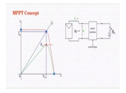
Now consider this modified figure  $R_T$  is the resistance seen across this terminal viewers on the PV module side so view from here the terminal resistance is called  $R_T$  and that is what I am using for load line so this is the load line having admittance  $1/R_T$ . Now this IV characteristic of this particular PV panel let us say is like this and the point of intersection of the load line  $1/R_T$  line with the IV characteristic is the operating point.
