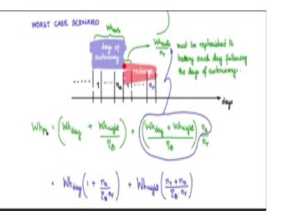
This is the standard requirement where the PV has to supply the day load plus the night load plus the battery charge and discharge losses apart from this it has to supply the energy required for the days of autonomy which is whatever D plus wait overnight so when the Sun power is not there both these has to be stored into the battery and therefore you have the F in the battery coming into the picture.
