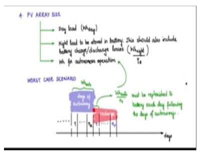
Let us see now how we go about sizing the PV array the PV array has to deliver rather words in the following way to the following loads the first one is the day load which we have called  $W_{hd}$  the second one is the night load, the night load is actually to be stored in the battery during the daytime so when during the daytime end the Sun power is present the PV array has to pump this much amount of whatever is where I was night load into the battery and the PV array or as.
