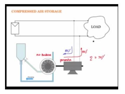
Another energy buffering mechanism is the compressed air storage mechanism, here the energy is stored the excess energy from the PV panel is stored in compressed air by virtue of the increase pressure, here again we shall use a motor which converts electrical energy into mechanical energy at the shaft and the shaft of the motor is connected to an air compressor the in compressor takes in the ambient here atmospheric air compresses it and puts it into a container through a non-return valve.
