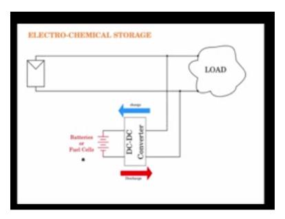
So generally in the case of a PV system we have a PV panel like this and that is connected to some load, energy is flowing from the PV panel to the load however we know that due to varying insulation the energy output of the PV panel is not constant throughout the day it keeps
