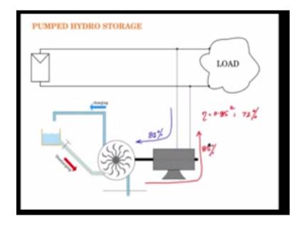
Another energy storage mechanism is called the pump hydro here the energy is stored by virtue of lifting water to a height and storing it as potential energy, so let me now show you the components that come within the system and then we will see the various modes that the charging mode and the charging mode this is a motor the electric power here will drive the motor and convert the electric power to mechanical power.
