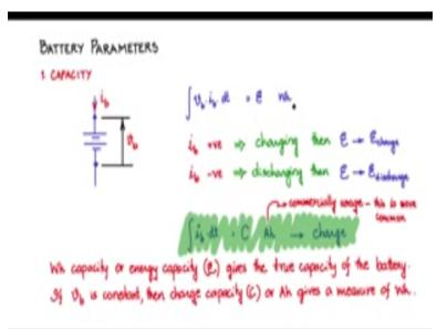
There are certain battery parameters that you should be aware of in order to select and specify for batteries one of the most important parameters is capacity of the battery what is capacity of the battery so let us consider this figure which gives you a picture of the battery symbol and these are the battery terminals let us say and then there is a current flowing into the battery positive terminal and that is called IB and let me mark the voltage across the terminals and we will name it as VB.
