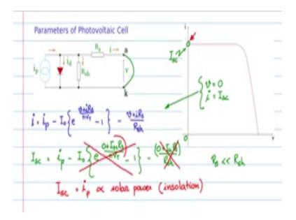
In this clip let us discuss the parameters of the photovoltaic cell for this let us have the model of the PV cell this is the equivalent circuit model of the PV cell we have the IT T photo current the diode part the shank non-ideality and the series non-idealities coming here and these are the terminal voltages and the currents of the PV cell let us have in place the IV characteristic of the PV cell 2 we will need this for our discussion.
