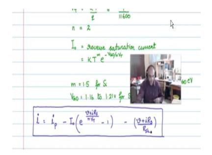
So these are the typical values using which you can get the reverse saturation current for a particular PN Junction device the entire model of the photovoltaic terminal current can now be written as IP is the photocurrent the directly proportional to the incident solar radiation  $-I^0$  to the power of V terminal voltage plus iR<sub>s</sub> by n VT- the current flowing through the shunt resistance which is given like this.
