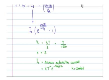
So this is given by the following relation K  $T^m e^{-vgo}/n VT$  the same n VT coming into the picture here where K is a constant which depends upon the dimensions of the PN Junction and also the material properties and  $V_{go}$  is numerically the equivalent band gap energy in electron volts so  $V_{go}$ is basically the forbidden the band gap energy which is  $V_{go}$  in electron volts.
