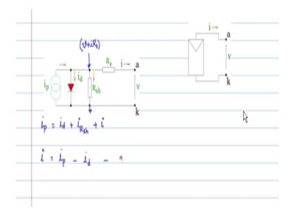
Let us clear someplace and position the equivalent circuit here the looking at the equivalent circuit the current Ip is equal to Id the diode current+ the current through the resistance R shunt+ the terminal current I if you consider this as the reference node the voltage at this node again can be seen that it is equivalent to V Plus this drop and this drop is having a potential which is positive here and negative here.
