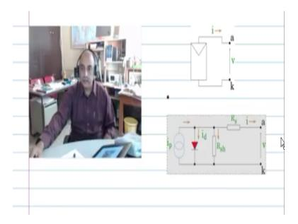
We have here a photovoltaic cell the symbol of a photovoltaic cell the terminal voltage V and the terminal current I that is supposed to flow out of the terminal a here is indicated and we also know we have seen before the equivalent circuit model of this photovoltaic cell and that is like this where you have this constant current source representing the photo current the photo current IP is basically directly proportional to the incident solar power.
