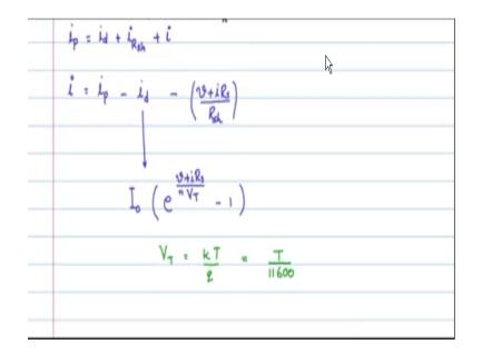
We know from the  $P_N$  Junction theory can be written as I not which is the reverse saturation current e ^ voltage across the diode which is nothing but V + iR<sub>s</sub> by an ideality factor n\*VT-1 so this is the equator antique equation for the diode it comes from the  $P_N$  Junction theory which you will find it in any electronics the injunction chapter typical difference would be the integrated circuits electronics by Millman and how caves.
