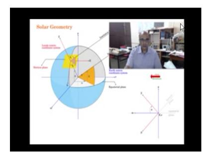
In order to estimate the insulation in kilowatt/m<sup>2</sup> and the hedge the energy in kilowatt hours/m<sup>2/</sup>day at any given point on the surface of the earth we shall use the help of solar geometry solar geometry is nothing but the spherical coordinate system but if as it also involves the position of the Sun in relation to the earth it is generally referred to as solar geometry apparently the figure here looks complex but it is not as complex as it looks.
