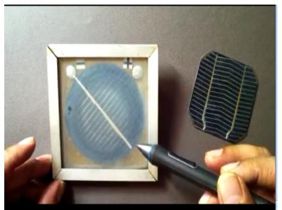
Here is an example of a poly crystalline photovoltaic cell this is the top layer which is the N type part of the PN Junction the bottom layer is the p-type and the p-type substrate metallization so normally what you would see is that then-type metallization are joined together and then that would be connected to the minus terminal and the p-type metallization would be connected to the plus terminal.
