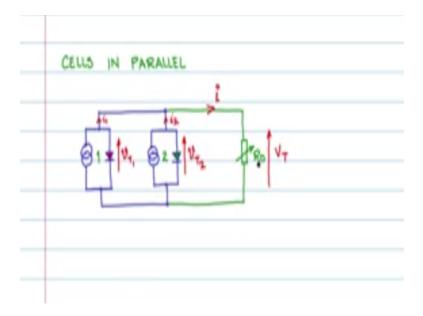
I can replace the PV cell symbol with the current source diode model the idealized currant source diode model so that we will be able to understand the operation much better right this completing the replacement we see cell 1 replaced by the current source and this red color diode cell 2 replace by this current source and the green colored diode this is paralleling to PV cells in parallel along with an external resistance R0 which has a stern load.
