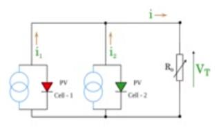
This is the circuit of 2 PV cells in parallel let us zoom in and it is clear that we have these two cells PV cell 1 and PV cell 2 in parallel with load or not this here is I1 which is the sourcing current from cell 1 I2 is the current from cell 2 I1 and I2 add up to give you I which flows through the external load R0 and VT is the voltage across the terminals of T cells parallel cell system.
