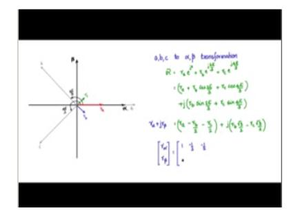
Now let me draw the  $\alpha\beta$  axis now I have  $\alpha\beta$  axis on that I will superpose the A B C axis and let me take a vector RA vector RB and RC in this fashion so this is just an arbitrary vector so Rea is along the y axis RB is along the B axis RC is along the C axis now our job is to convert the ABC vectors this could represent IA IB IC or VA VB VC so any arbitrary ABC vectors to  $\alpha\beta$ coordinate system.
