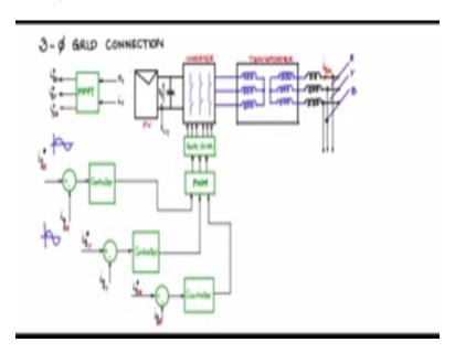
So this in this 3 phase grid connection system we would like to replace all these control blocks and we would like to have all the variables in the control, controller region as DC. How do we do that? Because all the signals that you are sensing are AC signals, how to go about doing this transformation.
