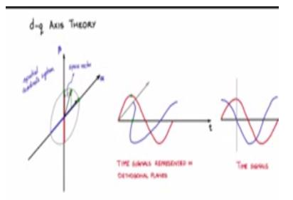
To do that we will discuss this dq axis theory there is this dq axis theory whereby it is a transformation principle where you can convert AC signals into DC AC sinusoidal signals into DC and then operate upon the DC values and then back again transform it into the AC domain where they will become AC signals, so this process of transforming from AC domain to DC domain DC domain to AC domain is what is popularly known as dq access theory which we will see now.
