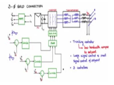
Let us now discuss the three phase grid connection of PV along with the control blocks, now consider this PV, PV module which is connected an inverter now I am starting with the three phase grid connection later on I will discuss the single phase grid connection actually if you see the three phase grid connection is much more easier than single phase grid connection therefore I have kept the single phase grid connection discussion to a later point in time.
