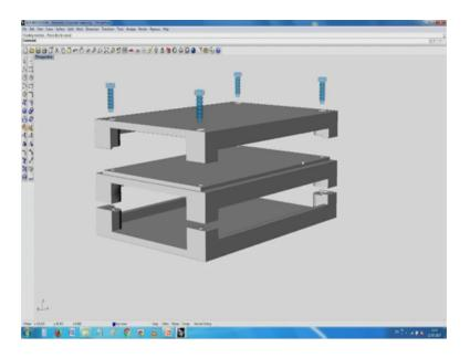
So, you see here things like the center portion or this one is the printed circuit board. For convenience I have put for you know holes in the corners advantages of being it is it has been made intentionally stack able you can stack them one over the other and is what when I was talking to you about building a library of components.
