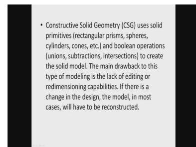
Use solid primitives, prisms, spheres, cylinders, cones and Boolean that is union subtraction and interaction to create the solid model. A lack of editing or re-dimensional capabilities, if there is a change in the design, the model in the most cases will have to be reconstructed. They somewhat you call freely downloaded from the net package which I use comes from this, but then since usually we have done a real big goof will not a small adjustment I am more used to making the whole thing again.
