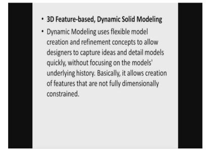
Next slide; dynamic modeling uses flexible model creation and refinement concepts to allow designers to capture ideas and detail models without focusing on the underlying history it allows creation of features that are not fully dimensionally constrained I thought.
