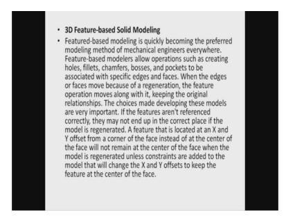
3 D feature base solid modeling is becoming the preferred modeling of mechanical engineers everywhere especially things which involve fabrication using conventional fabrication process.
