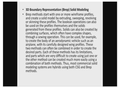
I will show you a last example at the end; Brep method starts with one or more wireframe profiles, create a solid by extrusion sweeping revolving or skinning. These profiles Boolean operations can be used the solids from these profiles can be made solids can be created by combining surfaces which have complex shapes through a sewing or welding operations used.
