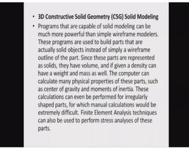
Solid modelers can be much more powerful than simple wire frame modelers. Actual solid objects instead of wire frame, since these parts are represented as solids have volume and given density have a weight and mass; computer can calculate many physical properties such as center of gravity and moments of inertia. Can even be performed for irregularly shaped parts for which manual calculation would be difficult. Finite element analysis techniques use to perform stress analysis.
