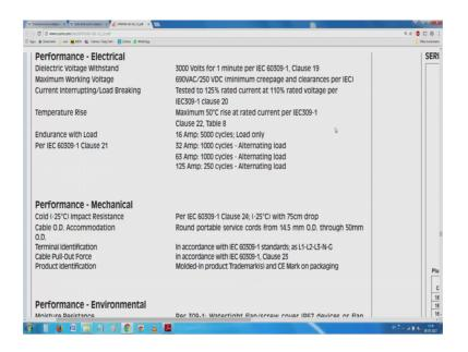
So, you seen this; electrical and mechanical performances are guaranteed, working voltage current interrupting a load breaking. 5000 cycles is directly endurance with some type of load alternating load means AC current haply we can break AC current. But there are little problem with a DC; DC tends to arc there is no arc quenching automatically.
