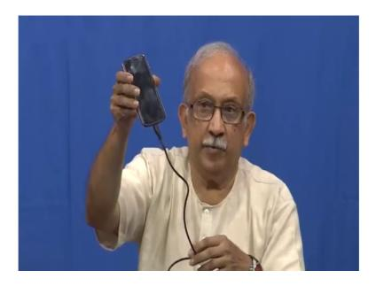
If have a mobile phone like this normally we connect this for connecting it to the what you call peripheral of the other side, but it has a small also called the OTG cable where the other side has a first connector the female part of it. So, if you have this now any of these devices can directly be plugged into the phone.
