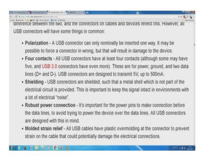
Metal shell just not part of the electrical circuit is provided. Keep signal in tack in the case of environments with lot of electrical noise. So, it is built in that the outside world.
