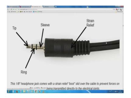
Most important thing here to when a connector wants to a board or a cable electrical connections tends to be fragile. It is typical to provide some kind of strain relief to transfer any forces acting on that connector to more mechanical sound object than the fragile electrical connections. So, I am sure all of you know about this 3.5 mm cable jack which we use in your headphones.
