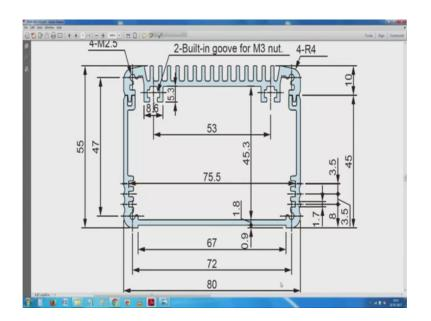
Ah now see something. So, we have a lot of details about how to assemble that nut, end at the bottom issues about the groove. And where the several other think and sit here one them is the printed circuit boards can sit here or you can have a HRC plate like thing which can sit here. So, lot of details about the groove and all and then yesterday if you remember I spoke to you.
