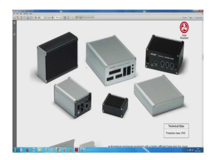
They are about the same; you know see here heat sink aluminium enclosures; it is all possible catalogue are geared and most important in the corner; see something in the corner protection classes IP40; 0 is not protected at all against ingress of any liquids or any fluids and any air borne any other materials.
