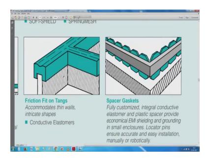
So, we have here friction fit friction fit means nothing, but just push it and then it squeezes itself on that on the edge of the enclosure then fully customized integral conductive elastomer plastic spacer and so on blah, blah, blah, all the stuff is available from multiple manufacturers. So, it is for you to decide what you would like to have and seen this you have clips to hold it and place and so on.
