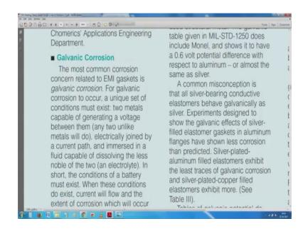
What is galvanic corrosion? For galvanic corrosion, a unique set of conditions; 2 metals capable of generating a voltage electrically joined by current and immersed in a fluid capable of dissolving the less noble of the 2 an electrolyte.
