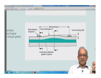
I mean a failure in a gasket ends up with a flooded crank case. So, a water ends up with you know small leakages will be there which go into crankcase and these will get circulated and then normal cases, there is no problem because once in a while I think routinely you check these things. So, as you go down you see you have this beautiful thing know where the bolt is spaced where it full force is there is, but in between we have the problem of things failing a little.
