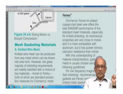
So, typically you are likely to see all this. So, ferrex tin plated copper clad steel wire offers a best EMI performance.
