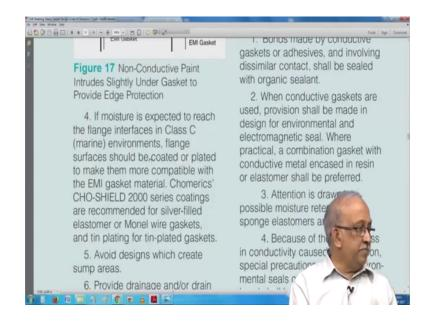
So, we have this class (Refer Time: 11:48) and if moisture is expected to reach the flange interfaces in class C marine; flange surfaces should be coated at to make them more compatible EMI and so on and so on there is a huge amount of how to deal with all these situations.
