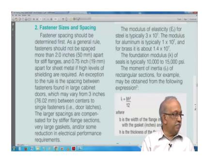
This is fortunately you know this equation does not look. So, threatening saying how much does the flange deflect fastener sizes spacing as a general rule should not be spaced more than 2 inches for stiff flanges more than twenty mm for sheet metal if high level of shielding are required.
