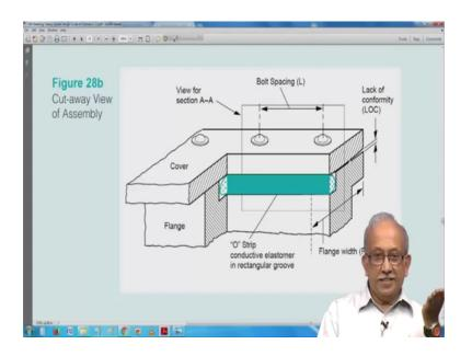
See here; so, you have bolt spacing and then you have an O strip conductive elastomer in a rectangular groove is a small errors can happen here lack of conformity to avoid this lack of conformity they will try to give the milling cut.
