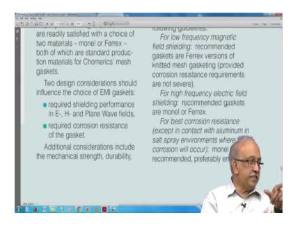
For low frequency magnetic field shielding recommended are ferex versions of knitted mesh high frequency electric field and so on first best corrosion resistance because who meant to have gasket we all this.
