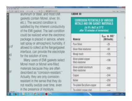
The thing is all this have been developed saying; how to apply these materials. So, you have here saying corrosion potentials of various metals and EMI gasket materials.
