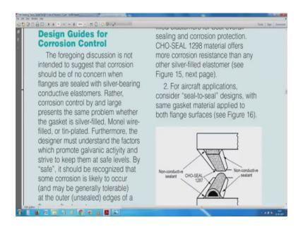
So, we have this very important thing corrosion control by and large present the same problem whether the gasket is silver filed monel; wire filled or tin plated furthermore designer must understand the factors which promote galvanic activity strive to keep them at safe level should be recognized some corrosion is likely to occur. So, seal to seal and so on nonconductive. So, on huge amount of data is available.
