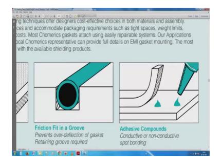
You see this know; we have adhesive non conductive spot bonding and friction fit in a groove and you see any number of robotically dispensed form in place conductive elastomer.
