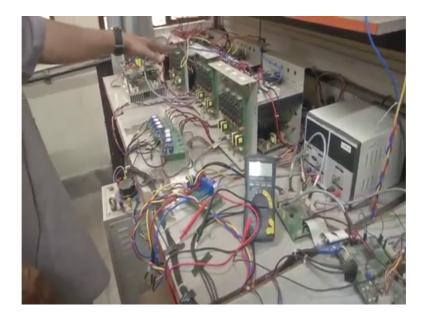
So, we have a c shaped what you call us support. Then we have this so called heat spreader, then the devices are all mounted there. And then it is easy for us to understand analyze and it is not tightly packed. So, start from here, then they whole place you see here these are the capacitors and that link voltage what I was talking to about link current So, they try their best to put whatever they can do and then see that the basic technologies proven.
