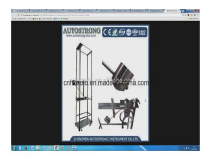
So, actually does not fall vertically at the bottom you have seen the mechanism this one is something which holds a hammer from falling. So, this is a release mechanism this goes and hits the vertical plate and then there are sensor which will ensure that the total energy that is transferred is fully controlled.
