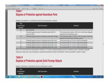
So, they have been using three numeral or two numeral designation which will ensure that first numeral talks about completely unprotected open pcb which I have shown you.
