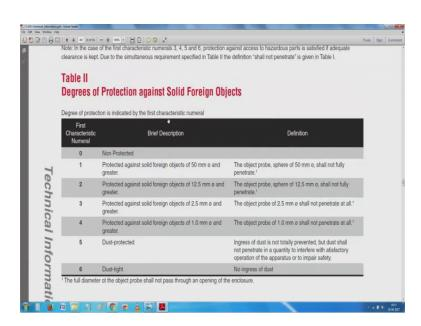
So, we have this once again know against solid foreign objects 60 millimetres pressure against 12 and half and then, against this thing and finally, dust protected and dust tight. This is where you would have heard about IP55, IP56, IP65, IP66 and so on. This refers to the first digit in that. So, both we have seen from inside to outside and outside to inside also.
