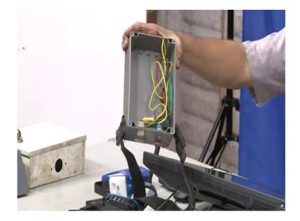
These are all meant for both indoor as well as outdoor uses. You notice here is, it is a polycarbonate or PVC enclosure. One of the things you see is elaborate arrangements have been made such that gasketing practice has been used. And then something related to this is also is that when you want to mount it, we have through and 3 holes here.
