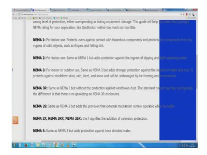
A little related to this is the IP classification saying the index of protection classes meant for other type of equipment where you have a 2 and 3 number system all of us are familiar with probably the IP 55 which is commonly used and then we have IP 56, IP 66 and finally, IP 67.
