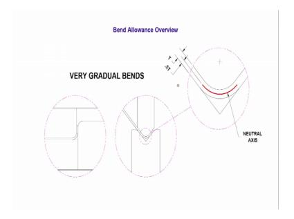
So, you have made things which have a very large gap here a gradual bend neutral axis is exactly 0.5.
