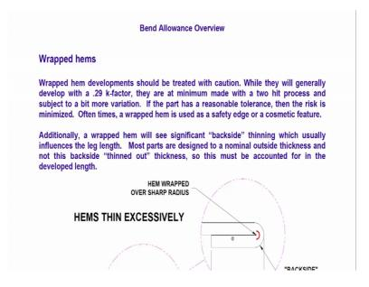
So, if you have completely closed wrapped hem developments should be treated with caution while they will generally develop with some 0.3 k factor they are at a minimum made with a two hit process and subject to a bit more variation. The part has reasonable tolerance then the risk is minimized.
