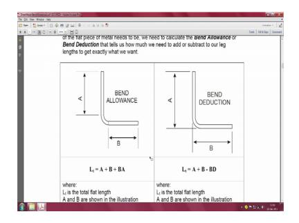
Instead here this is more related to if you take the internal dimensions minus the bending radius how do add a bending allowance where in the case you want take the external dimensions add the external dimensions and then you remove the internal dimensions.
