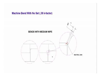
You see here bends with a medium wipe and you see here there is a smooth radius here in this corner, one of these limbs has a smooth radius so as we bend it with the this operation know will be slightly different from if it were directly done with the sharp radius and in this case you see here it could be something which is made at a different angle. So, there is a 135 mm angle here, this is 90 degrees, this is 135 mm. So, we have k factor which gives modifying all the time.
