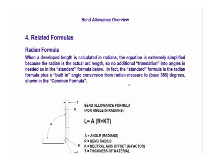
So, when you go down they try to come to the, can we have a formula when a develop length is calculated in radians. So, equation extremely simplified because radian is an arc length. So, no additional translation into angles is needed as the standard formula below. In fact, the standard formula is the radian formula plus a built in angle conversion from radian measure to base 360.
