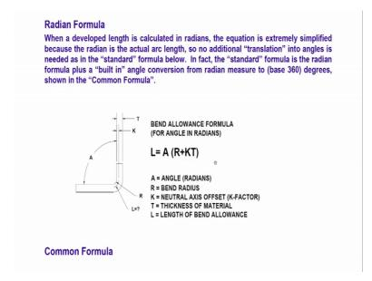
While this is nice for us probably from a physics point of view the reality is that we need to mark them in decimal millimeters. So, we have a height gage where the height gage somebody has to put the sheet that needs to be formed against a vertical surface and then do that in that case taking about things in radians for angles in know it does not makes in, but here it is about a is the angle in radians and then how to come back to making things understandable.
