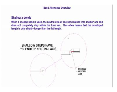
Here typically this is much less seen that know suppose is only one thickness offset. In this case the neutral axis is likely to not have too much of additional affect. So, here length is only slightly longer, when that talk about slightly longer it is probably not even measurable it should be the order of 0.05 or 0.1 millimeter long and then it does not matter because the limbs themselves know are the alter of limbs are so small.
