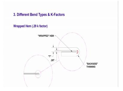
So, we see here a completely bent over 180 degree bend. So, can we actually make it flat some condition is depending on the softness of the material, the reality is that usually though it is not easily visible a small gap will be left there in this case you know it is given approximately one fourth of the thickness, a little over one fourth of the thickness.
