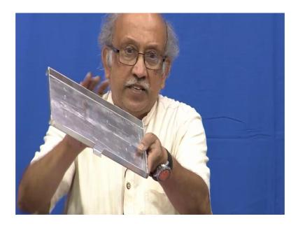
Exactly for this reason I brought you this, this is a wall mount bracket for what is called a cabin fan. So, this is whole thing we will get held on to the ceiling and then at the bottom we have an adaptor this is the bottom adaptor plate for that adaptor plate sits on this is and then we do various things and the whole fan, a fan base is locked on to this.
