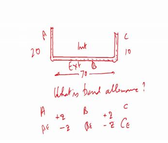
Movement add a thickness some other thing related to material behaviour that sent to the picture. So, this neutral axis does not change dimensions. So, when we are started with 100 mm. So, neutral axis inside it probably remains 70 here and then the neutral axis here know also remains 10 neutral axis here remains 20, but what does change is material here gets squeezed inside and here metal gets extended inside.
