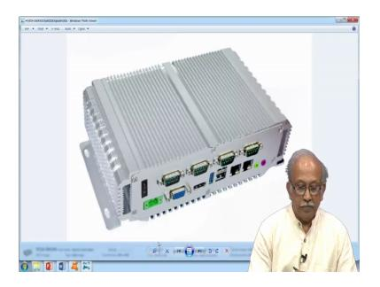
The casing usually outer most is made of aluminium just like I told you about the boxes oh we have a really beautiful example here it is a whole computer made fully out of extrusions you can see this there is a small screw here so; obviously, this piece is one extrusion and the sizes are also extrusions another small gap here you have seen there is a grows here then there is a slightly different type of orientation of the grows here plus there is a provision for us to attach there.
