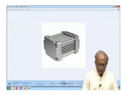
You have seen this you can say this type of construction in your pumps even a motor which has windings and this is iron core inside and you have copper outer most part is probably made of an aluminium extrusion and everything is assembled into it and you have bearings and their end plates and then probably if it is a pump you have an impeller or of its various other thing is just a motor.
