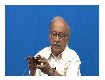
And the core of it is we have a transformer, why it is been made this way it is probably part of some rac equipment or something, where this directly gives an ac output and this ac output is treated to do various way. So, this is basically a very simple 230 volts to some wanted ac input thing.
