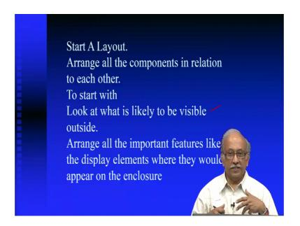
Not an easy life for all of them start a layout arrange all the components in relation to each other to start with look at what is likely to be visible outside, this is what I showed you a sample of the transmitter which goes with the wireless mic here. Arrange all the important features like the display elements where they would appear on the enclosure.
