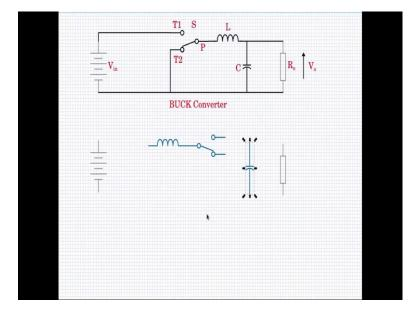
Coming to this BUCK converter here, we see that the energies flowing from the V in side to the V naught side. V in side is the higher voltage side and V naught side is the lower voltage side, now if we look at it in reverse from V naught side to V in side then the operation would look like a boost action, such a converter will be a boost converter.
