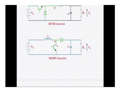
Now, this is a BJT. This BJT is one controlled switch likewise one could us a IGBT or a MOSFET controlled switches instead of a BJT. There is no problem in that any controlled switch for that matter will do. And another device is a diode. Now these two devices can be used to make up this single pole double throw switch. So, we can place the BJT in this fashion and series that with throw T1 and the diode can come along through T2.
