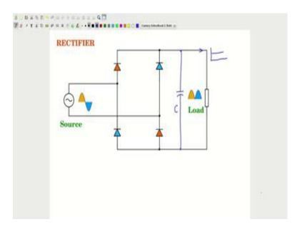
So, the total schematic of the rectifier is like this as shown. Now to this we have to connect a filter because this is a varying voltage we need to connect a filter it is a simple matter of connecting a capacitor like this as shown this is a capacitor c.
