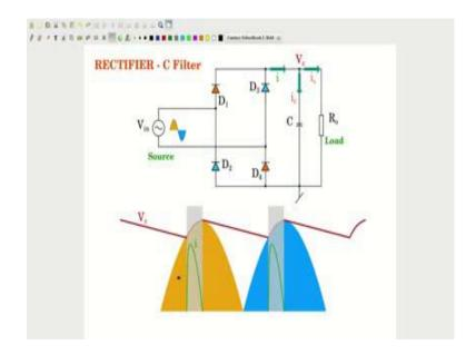
Now let us see the wave form in detail before that let us name the parts. So, the current that is coming out of the rectifier we will call it as I the current that goes through the capacitor as Ic the current that flows into the load r, not as I naught. Let us have this template this is the sine wave shape of each rectified half. So, this is the positive half of the input source this is the negative half of the input source rectified and placed in this fashion the uni direct load fashion.
