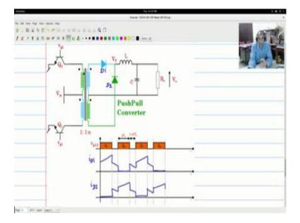
So, first let me take the diode current d 1 I will call this 1 as d 1. So, i d 1, during the time when Q 1 is on the diode d 1 will be conducting. So, it will take the same wave shape as the inductor current then the inductor current will actually, I will know going to put it dotted will go in this shape and then during the time when Q 2 is conducting actually the i d 1 current will not be flowing. So, I can safely say that it will be 0 during this time.
