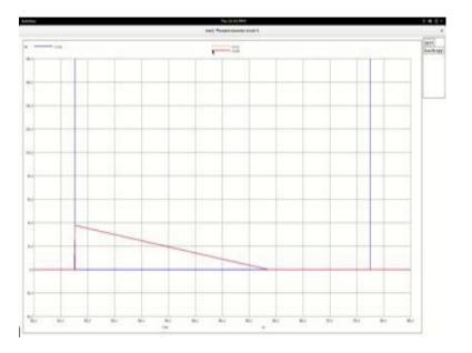
So, you see that it would be having a linear slope. The forward slope is also linear; the falling slope is also linear, because the voltage across the winding is text constant. Now if are decayed and because this is a less than 50 percent duty cycle this would have taken the same time to come down to 0.
