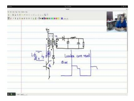
So, as you we can see this is the lossless core reset type of forward converter. There is one problem in this and that is we issue of leakage inductance. So, there will be some leakage inductance here. Leakage inductance means that that portion of the flux that is not coupled across between the two points and we mentioned and we discussed that this will be 1 is to 1 is to n and both the primary and the demagnetizing winding will be tightly coupled.
