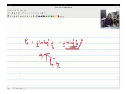
Another aspect is that the power dissipation are the power dissipation in R, the energy which is stored in the magnetic in the magnetizing inductance is half L m i max square. Now, this energy has to be dissipated with in R at this cycle. So, into t s this is the energy in joules by t s every cycle this energy has to be dissipated will give you the power dissipation R which is half L m i max, i max square into f s notice that the power dissipation in R is independent of that value of r.
