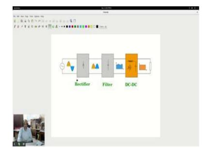
Consider a load such as this. This load is supposed to get only a DC voltage. The DC voltage can give by a DC source such as this. The DC source that we have used is a battery, however the battery and the load maybe incompatible. For example, the battery maybe a 12 volt battery or 24 volt battery or 48 volt battery and the load maybe a 5 volt load. In such a case the battery cannot be directly connected to the load which expects of high volt.
