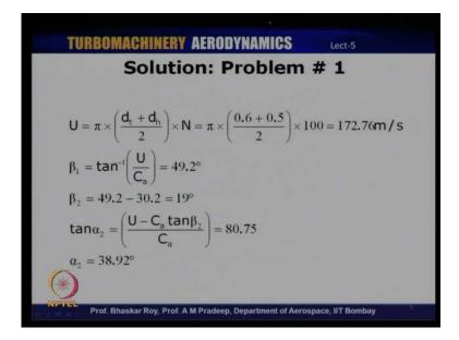
So, let us begin solving this part as well. So, what is given to us is the mean and we given the tip and hub diameters. The tip diameter is given as 60 centimeter and the hub
