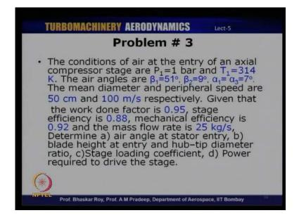
So, we have third problem statement here. The conditions of air at the entry of an axial compressor stage are P 1 is 1 bar and T 1 is 314 Kelvin. The air angles are beta 1 is equal to 51 degrees, beta 2 is 9 degrees, alpha 1 is equal to alpha 3 is equal to 7 degrees, the mean diameter and peripheral speed are 50 centimeters and 100 meters per second respectively.
