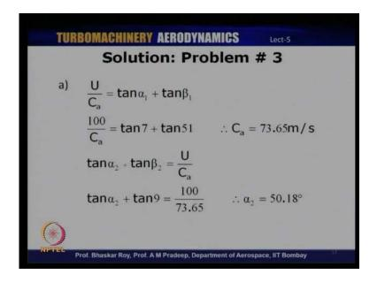
The first part of the problem is to find the air angle at the inlet which is alpha 2 at the stator entry basically for which, once you have constructed the velocity of triangle it makes it very simple to solve. From the velocity of the triangle you will see that the ratio U by C a should be equal to tan alpha 1 plus tan beta 1. This is basically because U is equal to C a times tan alpha 1 plus C a times tan beta 1, alpha one is known, beta 1 is
