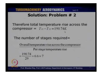
Therefore, the total temperature rise across the compressor is this temperature 522.5 minus 331.8. So, that is 190.74 Kelvin. This is the total temperature rise across the whole compressor. So, therefore, the number of stages required in this case will be the overall temperature rise across the entire compressor divided by per stage temperature rise that is 190.74 divided by 29, this is 6.6 and that has been rounded off to the next integer and that is 7.
