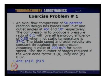
First exercise problem is an axial compressor of 50 percent reaction design that is the degree of reaction is.5 has blades with inlet and outlet angles of 45 and 10 degrees respectively. Compressor is to produce a pressure ratio of 6 is to 1 with an efficiency of 0.85 when the inlet static temperature is 37 degrees Celsius. The blade speed and axial
