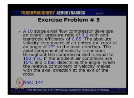
And the last exercise problem is a 10 stage axial flow compressor develops an overall pressure ratio of 8 with an isentropic efficiency of 0.85. The absolute velocity component of air enters the rotor at an angle of 27 degrees to the axial direction. The axial
