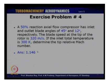
Fourth problem is a 50 percent reaction axial flow compressor has inlet and outlet blade angles of 45 degrees and 12 degrees respectively. The blade speed at the tip of the rotor is 320 meters per second. If the inlet total temperature is 300 Kelvin, determine the tip relative Mach number. In this case the Mach number is 1.146.
