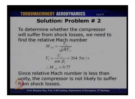
So, let us calculate the relative Mach number and then see if it is greater than 1. So, to determine whether the compressor will suffer from shock losses, we will need to find the relative Mach number. Relative Mach number is the ratio of the relative velocity to the
