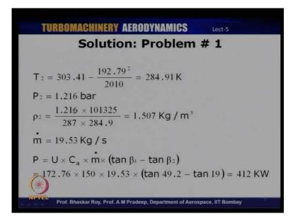
So, let us do that. Therefore, static temperature at the exit is T 2 which is 303 minus.41 minus 192.79 square divided by 2 into C p a that is 1005 that is 2010. So, this is 284.91 Kelvin. P 2 is the pressure ratio multiplied by inlet pressure, we get 1.216 bar. Therefore, row 2 is the pressure ratio which we have converted that into Pascals 1.216 into 101325 divide T by R t and R here is 287 into temperature 284.91. So, the density comes out to be 1.507 kilo grams per meter cube.
