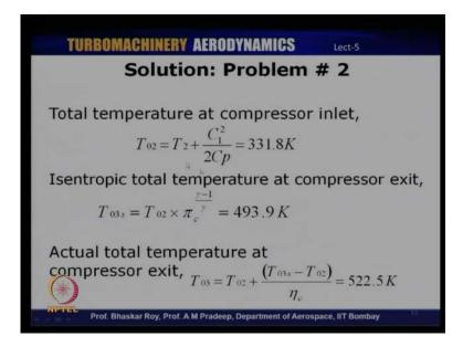
Total temperature rise we need to find the total temperature rise across the compressor and for which we will first find the total temperature rise at the compressor inlet, Which is this static temperature plus C 1 square by 2 C p, and that comes out to be 331.8 Kelvin and the isentropic total temperature at the compressor exit, which is T 03 s or the isentropic total temperature is equal to T 02 multiplied by phi c rise 2 gamma minus 1 by gamma this is 493.9 Kelvin.
