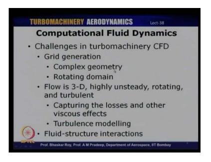
So, grid generation is an extremely involved process in turbomachinery flows plus the fact that we also have a rotating domain. The rotor blades are rotating and the rotating flow goes into the stator and which is stationary. So, how do how do you actually take this into account how do factor the fact that there is a rotating domain which is present in turbo machinery flows.
