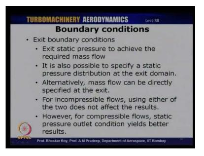
and but I say I mentioned for low speed incompressible flow it should not really matter whether you are specifying static pressure or mass flow rate and it is also possible that one can specify a static pressure distribution at the exit rather than just an average static pressure, one may also want to be a little more accurate, one can simulate a static pressure distribution as well at the exit.
