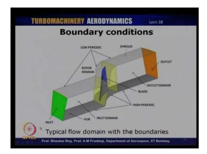
So, this is the typical flow domain with the boundaries I have shown. This is compressor blade here we have a low speed compressor blade the flow enters through the blade domain and here we have seen relating only one blade and since all the blades are identical we will have to set what are known as the periodic boundary conditions.
