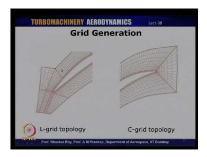
And let us take a look at 2 other grid topologies the L-grid and C-grid. This is the L-grid topology very similar to a J-grid, but just that in a J-grid one had a section here and this is basically the L-grid topology that you can see and this is a typical C-grid topology you can see that unlike the multi-block here multiple number of blocks here you have only 2 blocks which have been provided and this is the typical C shape that you get and that is why it is called a C-grid topology.
