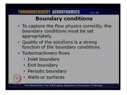
So, basically boundary conditions are essential in capturing the flow physics correctly and appropriately and; obviously, the quality of the solution that you get is a very strong function of the boundary condition itself.
