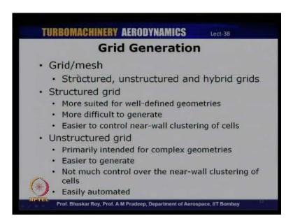
Now grid is the discretisation or grids are used for basically discretizing the domain and there are different types of grids or meshes which are available and which can be used. These can basically be classified as structured grids, unstructured grids and hybrid grids.
