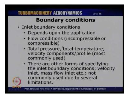
So, if you have to set inlet boundary conditions it; obviously, depend upon the application itself which depends upon the flow conditions whether it is incompressible or compressible, the most commonly used boundary condition for the inlet is this a set of predefined total pressure at the inlet, total temperature and the velocity components or profile at the inlet.
