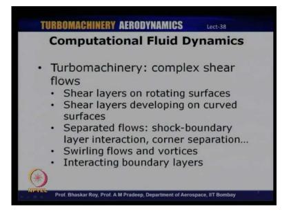
Now turbo machinery involves; obviously, very complex shear flows which involves shear layers on rotating surfaces on the blades. Shear layers on which are developing on the curved surfaces again on the blades, one may have separated flows which could be because of shock and boundary layer interaction or corner separation or during stall. Shock boundary layer interaction being when it is transonic case.
