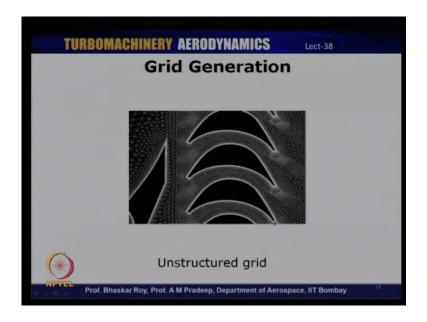
And this is a typical unstructured gird and you can see that the grids are not in a particular fashion. And they are relatively random and this is a typical example of an unstructured grid. These are unstructured grids you can see that immediately that not very easy to control the clustering around the blades where you would like to simulate the boundary layers as well.
