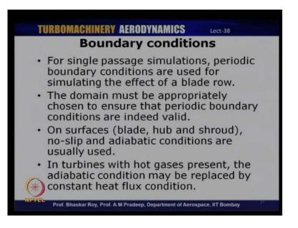
Now, for single passage simulation like the one I have just showed periodic boundaries are used for simulating the effect of a blade row and it is necessary that one appropriately chooses this domain, so that periodic or periodicity is indeed valid. And on the surfaces like the blade or the hub or the shroud it the standard boundary conditions like no-slip and adiabatic conditions are used.
