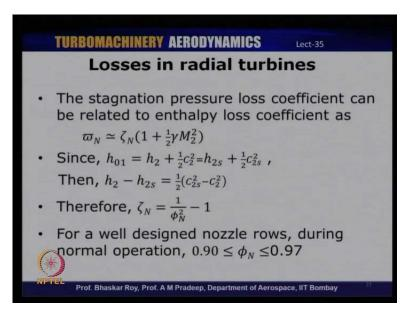
And you can actually relate some of these different loss parameters; the stagnation pressure loss coefficient is approximately related to the enthalpy loss coefficient through the Mach number. So, omega N is approximately equal to zeta N into 1 plus half gamma by 2 into M 2 square, where M2 is the absolute Mach number at the rotor entry, which is basically related to C 2 and the temperature at the rotor entry.
