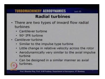
We will look at two distinct varieties, which have been used over the past many years and these are the cantilever type turbines and the 90 degree IFR or inward flow radial turbines. So, these are two distinct types of inward flow radial turbines, the cantilever type turbine and the 90 degree inward flow turbine. Out of this, of course, we will spend the rest of the lecture discussing primarily about the 90 degree inward flow radial turbine or IFR turbine.
