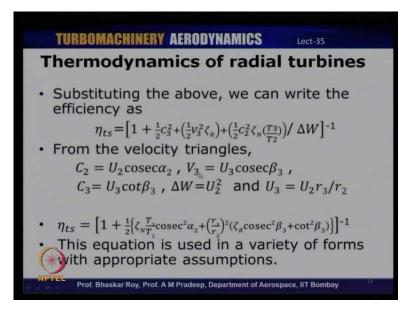
So, with this definition of the passage enthalpy loss, we will substitute these in the previous expression, that we have written down, that is, for the total to static efficiency and then, if we substitute these values here, we will get the revised formula definition for the total to static efficiency as 1 plus half C 3 square plus half V 3 square into zeta r plus half C 2 square zeta n into T 3 by T 2 divided by delta W raise to minus 1, so, or delta W divided by this.
