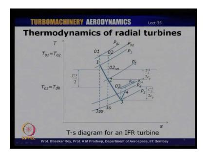
So, a T-s diagram for a typical inward flow radial turbine would look like this. Let me explain the different components associated with this particular T-s diagram. As we have seen before, station 1 is the nozzle entry, station 2 is nozzle exit, 3 correspond to rotor exit and 4 correspond to the diffuser exit.
