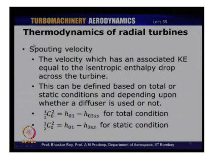
So, this is basically known as the spouting velocity and it has primarily been used in the hydraulic turbine context, but sometimes it is also referred to for normal gas turbine applications as well.
