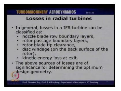
So, in general, if you look at the different sources of losses, let us be specific for an inward flow radial turbine, then the various sources of losses can basically be the nozzle blade row boundary layers, the rotor passage boundary layers, then you could have tip leakage or tip clearance effects at the rotor exit, the disc windage, that is, the rotor surface itself can lead to certain amount of windage losses and the kinetic energy loss at the exit.
