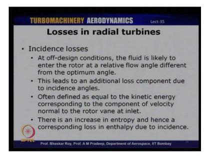
So, at off-design condition, the flow is likely to enter the rotor at a relative flow angle, which is different from the optimum angle and this leads to an additional loss component due to incidence and this is often defined as equal to the kinetic energy corresponding to the component of velocity normal to the rotor vane at the inlet.
