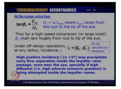
Let us start at the beginning of the centrifugal compressor, where you need to create the inlet flow and the inlet vane shape. The flow is coming in with tan beta 1 which is C a 1 by U 1, as we saw in the velocity diagrams. U 1 is of course, is omega into r of the eye which as we saw varies from root to the tip of the eye.
