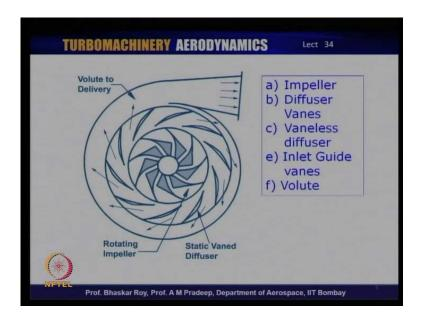
Now, the centrifugal compressors which we are looking at, typically has a rotating impeller, which is normally, called impeller over the years, and of course, the static vanes at the exit to the impeller, and these are two necessary ingredients of a centrifugal compressor.
