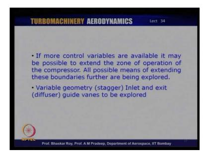
More control variables, if they are available, it may be possible to extend the zone of operation of the compressor, and sum of the possibilities are variable geometry, inlet guide vane and even variable geometry exit diffuser guide vane, which is very difficult because the flow there is at high speed, but inlet guide vane variable geometry is indeed quite possible.
