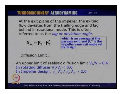
Then, at the exit plane of the impeller, as we have seen, in the flow actually, it has the two vanes. One of them is essentially a trailing edge and the other one can be called the leading edge. So, depending on the direction of rotation, the flow often has a tendency as we have seen, deviate from the trailing edge, because of this deviation, of course, we had the slip and the name slip comes from the fact that the flow so to say, slipped from the trailing surface of the blade.
