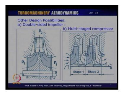
Now, a double-sided impeller is essentially one in which the flow is actually being brought into the centrifugal compressor from two sides. This is essentially done to increase the mass flow through the centrifugal compressor and as the mass flow through centrifugal compressor is somewhat restricted by its inlet, which is smaller than its a outer diameter.
