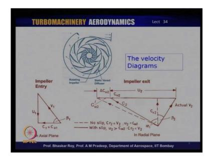
Now, let us take a look at something that you have done in great detail is the velocity diagrams that typically are operative at the entry and exit of the impeller; impeller, being of course, the most important element that needs to be designed. Now, at the impeller entry, as you have done the flow often is expected or allowed to come in axially.
