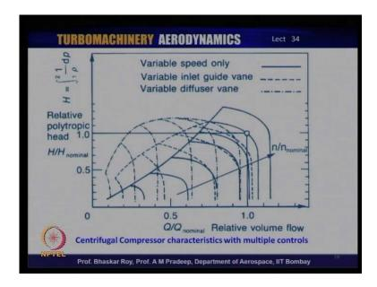
If you do have a variable geometry inlet guide vane, you can extend this stall line further to the left, and extend the operation of the centrifugal compressor. This is a typical centrifugal compressor characteristic map and you can extend it far to the left.
