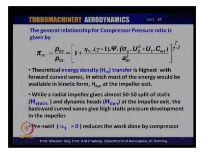
The general relationship of the compression pressure ratio is as you have done earlier depends on the efficiency. It depends on the blade loading, the losses, and the slip factor and of course, the velocity triangle that we have done before. As we have seen, the theoretical energy density transfer is highest in forward curve but, it has all kinds of other problems and hence normally is not used in modern centrifugal compressor especially in aero engines.
