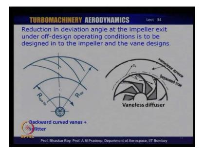
The choice of the diffusion process after the impeller is, you can have a vaneless space, so the vaneless space, we are talking about is completely extended over the entire vaneless diffusion area. You get a broader mass flow but, you have a somewhat lower
