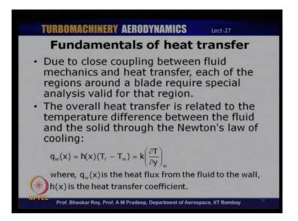
So, analysis of the flow around a blade requires special analysis which is valid for that particular region. For example, if you are looking at laminar flow that is leading edge of turbine blade, then one can analysis the heat transfer through a laminar boundary layer and has been transition and go to the later part of the turbine blade. The boundary layer is Turbulent and heat transfer through that boundary layer is quite different.
