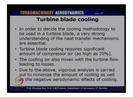
So, just to summarize the various points regarding with reference to blade cooling methods, needless to say of very strong understanding of the heat transfer mechanisms is essential because cooling a turbine blade is essential heat transfer problem, of course, there is also strong coupling of heat transfer with the fluid mechanics here.
