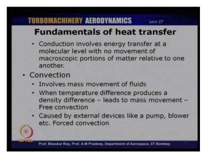
Conduction as I mentioned is energy transfer at a molecular level. There is no mass movement or macroscopic movement of matter relative to one another. Now, the other mode of heat transfer is convection, and convection is something that involves motion, mass motion of fluid and it is not something which occurs on a molecular levels. So, there is much more than just molecular motion; it involves basically mass motion of fluids either liquids or gasses.
