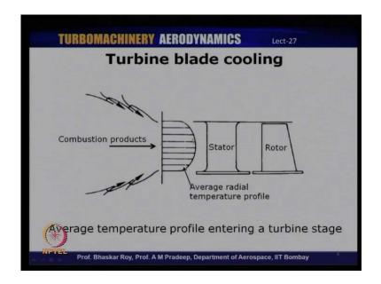
Just you give me some idea if you look at this particular schematic where we have an average temperature profile which has been plotted. This is an average radial temperature profile. So, this is a typical average temperature profile, radial temperature profile, that is, from the hub of the blades to the a shroud and combination products enter the stator typically with an a certain temperature profile.
