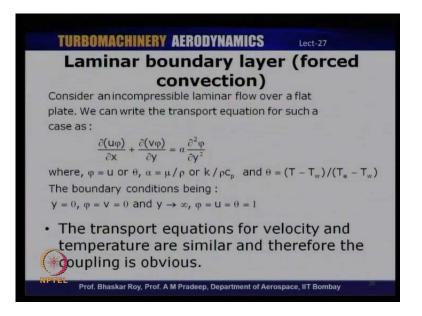
So, let us consider a very simple case of an incompressible Laminar flow over a flat plate. So, for this kind of an application, we can write the transport equation as del u phi by del x plus del V phi by del y is equal to alpha del square phi by del y square. So, here, phi could be either u or theta; alpha could be either mu by rho or k by rho C p and theta is the temperature differential t minus T w by T u minus T w.
