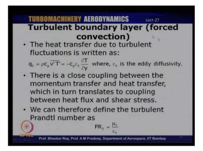
So, heat transfer to which is owing to turbulent fluctuation is can be written in the form of this equation, that is, q subscript t is equal to row C p into v prime t prime, and average of that the end symbol average of that this is minus C p into epsilon subscript t del t by del y which is at temperature gradient. Here, epsilon subscript t is the eddy diffusivity which is basically owing to the turbulent fluctuation which of present in a turbulent boundary layer.
