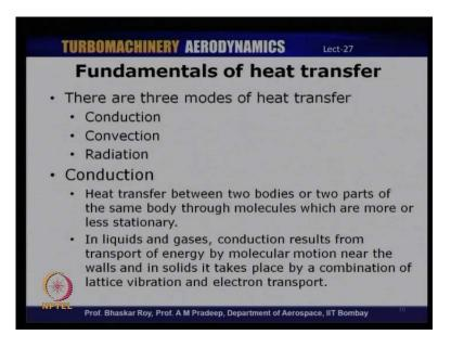
And so, and in the case of gases and liquids, conduction basically results from transport of energy by molecular motion near the walls, and in solids, it takes place by a combination of lattice vibration and electron transport.
