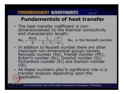
Now, this heat transfer coefficient that we have seen can be non-dimensionalized by the thermal conductivity. So, and that is through what is known as the Nusselt number. So, Nusselt number is the heat transfer coefficient multiplied by a characteristics line usually the god of the blade in these case divided by the thermal conductivity of the blade. This is also equal to l by the temperature difference t minus T w multiplied by del t by del y at the wall.
