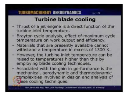
So, so with the gain in performance we have mechanical aerodynamics thermodynamic complexities which are involved in design and analysis of these cooling techniques and ah
