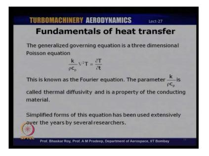
Now, this equation we can generalize and we can write a generalize governing equation in a three-dimensional Poisson equation form and which is basically stated as by rho cp del square t is equal to del t by the rate of change of temperature are with time. So, there is transient temperature term here. The temperature denser here and the parameter that you see here, that is, k by rho cp is known as thermal diffusivity which is again a property of the conductivity material.
