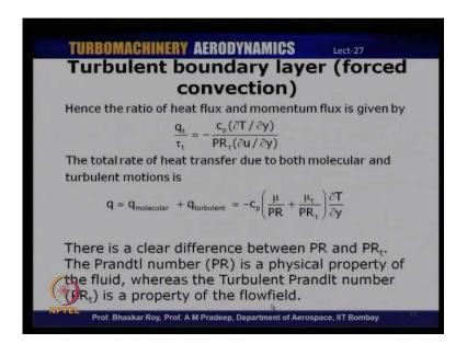
So, what is the significance of the Turbulent Prandlt number? We can express the ratio of heat flux and momentum flux as what is given here, that is, the heat transfer q t to the momentum flux is equal to the mines C p into temperature gradient and the turbulent Prandlt number multiply by the velocity gradient.
