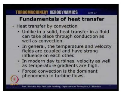
Now, in ah modern day turbine scenario, we, the coupling is even more significant because of the fact that velocity as well as temperature gradients are very high, and in that scenario, the coupling between the temperature and velocity fields will have a very strong influence on each other, and turbine blade which is and do which is being design, which has been design for cooling methods will involved forced convection and that is the dominant phenomenon of a heat transfer in turbine flows.
