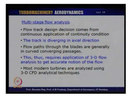
So, the modern turbines are analyze indeed through 3-D flow analysis techniques, and then you need to apply 3-D CFD techniques, analytical techniques that are available or whatever is made available to you, simple two-dimensional analysis would fall short of the requirements of modern turbine design. So, 3-D analytical techniques would need to be adopted very vigorously for modern turbine design.
