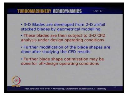
So, in summary, we can say, that the 3D blades are indeed developed or reconfigured or reshaped from earlier known two-dimensional airfoils, and then they are stacked by geometric modeling; modern blades are not stacked radially anymore. These blades are subject to intense 3D CFD analysis under design operating conditions. Further modification of the blade shapes are done after studying the CFD results.
