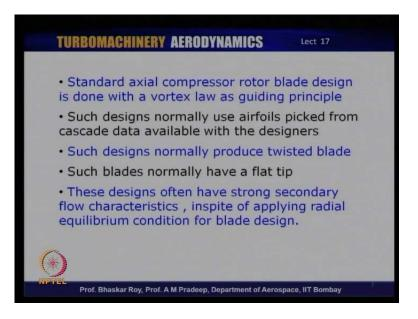
What happens is, a standard axial flow compressor blade shape is done with the help of some of the vortex law starting with a free vortex law, which we have done in great detail as the guiding principle. Now, that allows you to gated to the three-dimensional change in aerodynamic parameters. When you do that, the twist automatically comes into the shape. So, twist is there, even in what is called pseudo two-dimensional design methodology.
