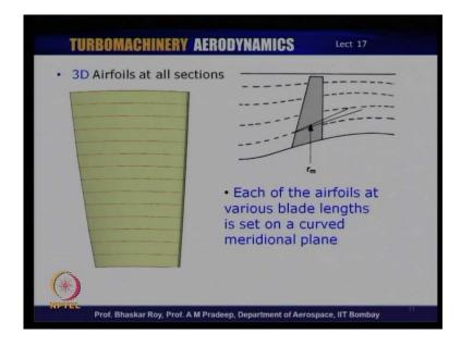
However, the more modern designers would like to see where all airfoils are essentially arranged in curvilinear surface. So, all the airfoils now, indeed all the way from root to tip, are three-dimensional airfoil. Now, geometrically you see it make sense, because, if you look at this picture, which we have seen before; this is the meridian path that we have talked about and this meridian path shows that it is not constant radius, radius here and radius here are different.
