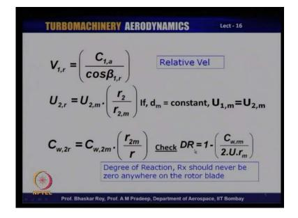
Correspondingly, the relative velocity of course, can be found out as per the velocity triangle using the values, that axial velocity and the relative velocity that we have found.
