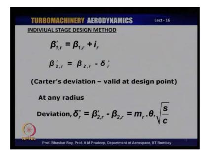
If you choose the incidence the way we were talking about, then your solid body of the blade would need to be set at an angle, which is then beta 1 plus the incidence and that becomes the solid incoming blade angle or the inlet blade angle at the entry to the blade.
