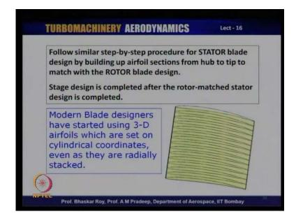
So, these stages often nowadays need to be gone through the CFD analysis. The modern designers often also end up using aerofoils, which are 3D aerofoils. That means, the
