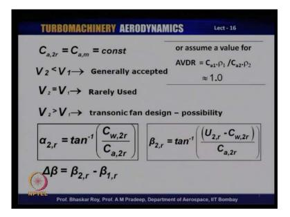
If we proceed with the steps, that we are going through we can now see, that one of the assumptions, that you may like to make at this stage for simple design procedure is that the axial velocity through the stage is remaining constant at that particular section. So,
