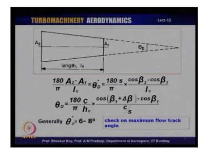
Now, some of these things are initially created with the help of some very simple considerations. So, what we are looking at is a simple conical annulus track. So, the track is annulus, if you remember. However, the construction of the track can be considered to begin with a conical one.
