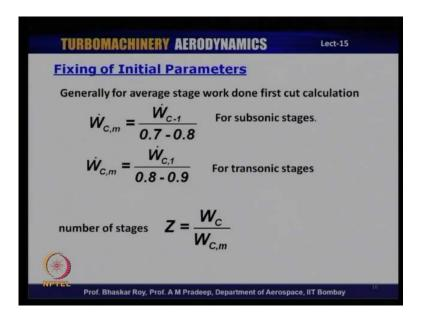
And then, of course you need to fix the initial parameters that mean, the work to be done by the individuals stages. A conventional method is, if you have in a subsonic stage, you can try to pump in certain amount of work; if it is transonic stage you can pump in certain amount of work.
