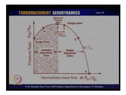
So, this is the kind of compressor characteristic, that you have done before and we will take a quick look at this characteristic map. Now, this line, that you see, is the characteristic of the compressor at its so called design speed.
