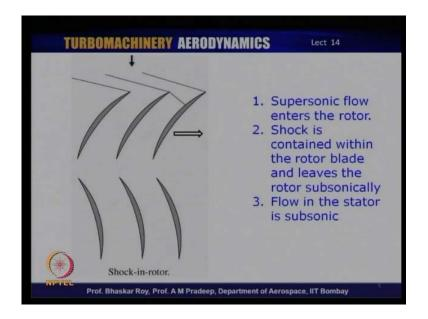
Now let us likely a look at various possibilities that I have just been talking about. The possibilities is indeed that the shock is only in the rotor that means only the rotor has gone supersonic which essentially means that the flow coming into the rotor is supersonic and then you have a shock standing in front of the blades.
