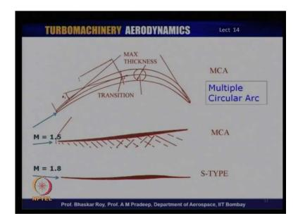
On the other hand, the further development of double circular arc created the multiple circular arcs. Now multiple circular arc, as the name suggests, has more than two arcs in creation of an airfoil you can have one circular arc here, another circular arc here on the same surface, on the suction surface you may have one circular arc here another circular arc arc over here. So you may have minimum of four circular arcs in creation of an airfoil.
