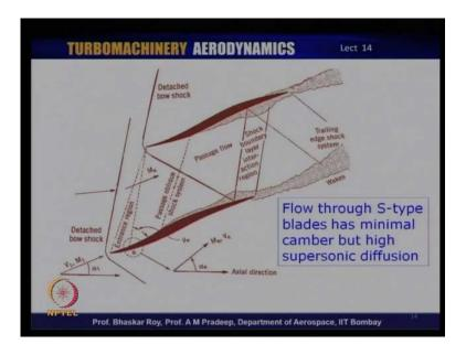
If you take the S type blades which have very high Mach number of the order of 1.8 or so as we can see in this shock structure, one of the shocks is again going out, the other shock which is gone inside the blade, now actually hits the next blade somewhere near the trailing edge. Which means on this blade, all the way from leading edge to almost near the trailing edge to the flow is actually supersonic.
