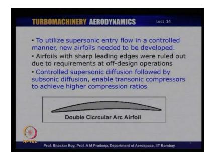
So let us take a look at some of these new kind of airfoils. The first kind of airfoils that was created is simply called double circular arc airfoil. Now it actually is called double circular simply because it as two circular arcs, one circular arc of the pressure surface and another circular arc of the suction surface. So the entire suction surface and the entire pressure surface each are made of one circular arc and two of them together create double circular arc airfoil.
