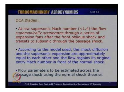
The DCA blades, the supersonic Mach number is normally less than 1.5, 1.4 typically by 1.5 you would need to use MCA blades and in DCA, as we have seen in the flow accelerates through a series expansion fans, after the front oblige shock and then transits to subsonic through passage shock.
