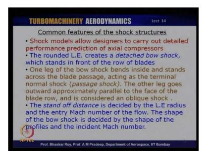
Now let us look at the common features of shock structures, the shock models allow the designers to carry out the detailed performance prediction of the axial flow compressors. Remember what we have seen are essentially shock models. During actual operation it may or may not exactly operate as per those models. However experiments have clearly
